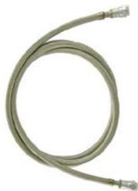
SICERA® Cryopumps come equipped with flexible helium gas lines in 82 feet (25 meter) lengths, while Marathon® CP Cryopumps come standard with flexible helium gas lines in lengths from 10 feet (3 meters) to 66 feet (20 meters). Gas lines terminate in size 8 female coupling halves for quick connect and disconnect to/from the cold head and compressor and are also available with one end at 90°.
